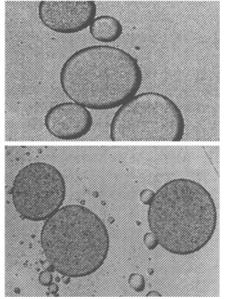
Placing the surfactant in the aqueous phase prior to mixing fails to produce good quality multiple droplets. Small 'specks' can be seen in the oil globule (Figure 1a) in contrast to well-defined larger inner droplets formed on addition of an oilsurfactant mix (Figure 1b). The corresponding average medium size values were 294.9µm (SE:10.75) and 176.52µm (SE:1.95).
